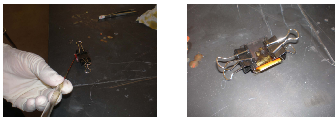
Figure 5. Adding iodide electrolyte solution
